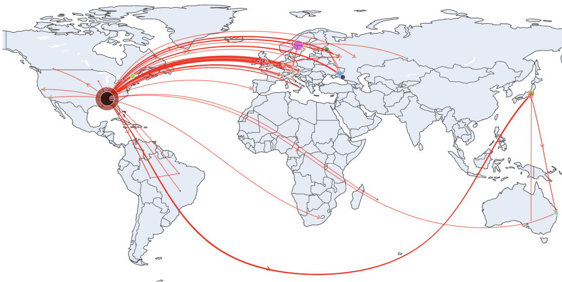
Figure 7.19.: Time-range 1: State before Pakistan's misconfiguration. The large black dot is YouTube's AS36561 which originates all shown AS-paths. All other dots represent ASes that are destinations of YouTube's routes.
